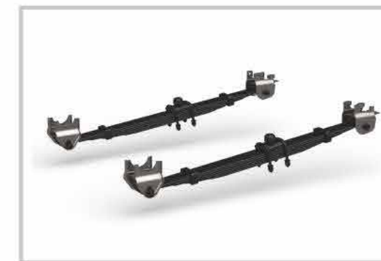
Strong front & rear suspension with added leaves
